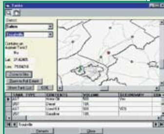
The above Windows® application displays storage tank locations and contents. Digital photos gathered in the field can also be stored with each feature.
