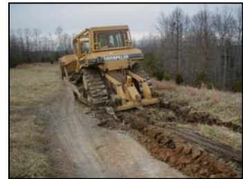
Stable, but highly compacted, reclaimed areas support grasses and shrubs, and often little else. Preparing the surfaces for trees requires excavating rooting zones with a backhoe ( left ) or ripping the surface ( right ). Both methods loosen the rooting zone for better seedling survivability and tree growth.
